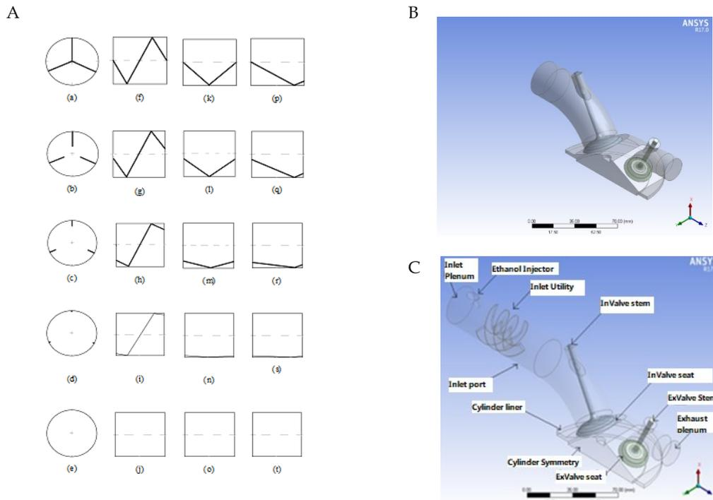
**Figure 3.** (A) Representation of radial blade profile and spiral pitch length for three cases for 30mm long inlet port utility with BRL of; (a) Blade through-15mm, (b) 10mm, (c) 5mm, (d) 2mm thick spiral, (e) plane connector, and (f-t) pitch length of 30, 60 & 90; (B) base model, and (C) model with inlet utility.
