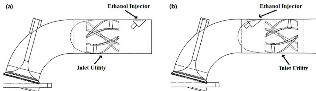
**Figure 2.** Port injection utility indicating; (a) Ethanol port injector and swirl generator blades, (b) Injector placed after the swirl blades
