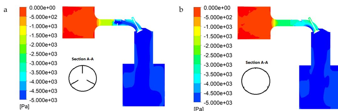
**Figure 7.** Pressure contour of flow through the intake port at 10mm valve lift with utility of; (a) 10 mm BRL and (b) 2mm BRL
