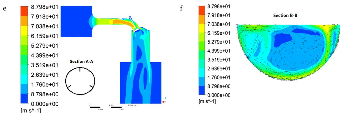
**Figure 6.** Velocity Magnitude on Cut plane 1 (symmetry of the cylinder) and Velocity Magnitude with Vectors on Swirl Plane 2 (45 mm from TDC) at 10mm Valve Lift for 90mm pitch Model with BRL of (a&b)15mm; (c&d) 10mm and (e&f) 5mm.
