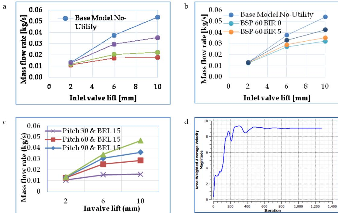
**Figure 5.** Mass flow rate for inlet modification design modeling of the Swirl Blades (a) Different BRL for spiral pitch of 30mm; (b) spiral pitch of 60mm; (c) different spiral pitch and BRL of 15mm; (d) velocity magnitude convergence on out-plenum.
