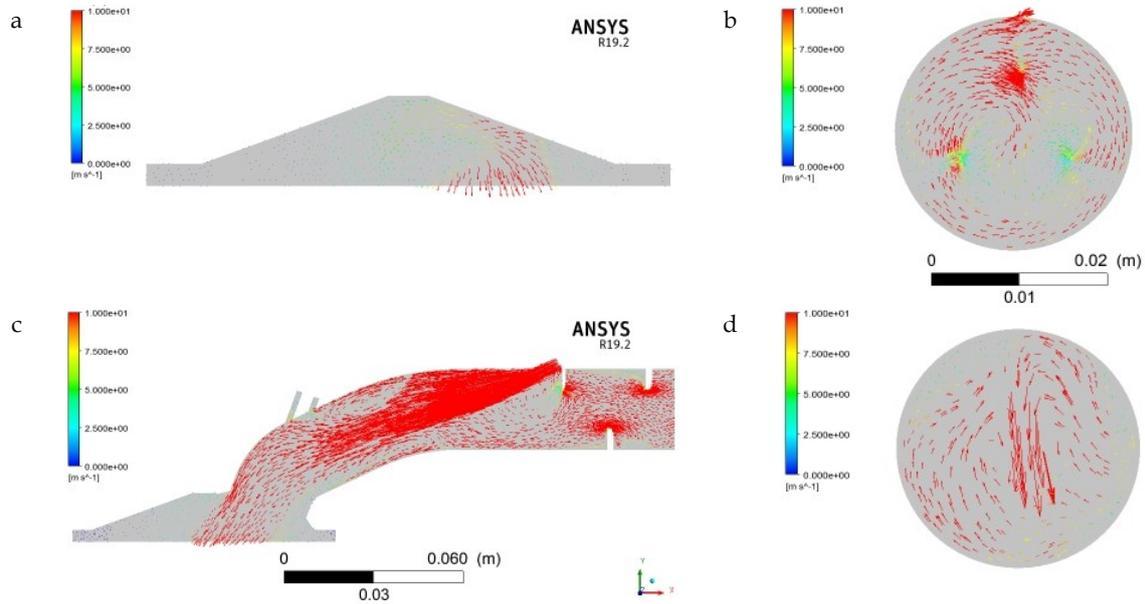
**Figure 4.** Velocity vector for Ethanol PFI simulation for inlet port with inlet utility at (a) cylinder cut plane; (b) exit of swirl blades; (c) inlet port; and (d) after injector
