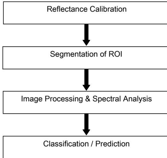
Figure 2. Flow diagram of hyperspectral data analysis process
