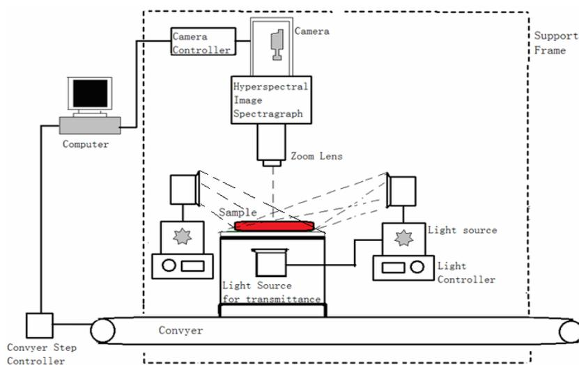
Figure 1. Configuration of a hyperspectral imaging system
