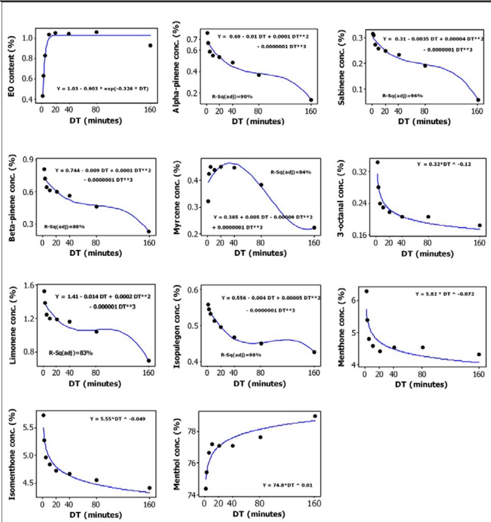
**Figure 6.** Plots of essential oil (EO) content and the concentrations of 10 compositions vs. distillation time (DT) together with the fitted Asymptotic, Power and third-order polynomial regression models. Equations of the fitted models are shown within each plot.
