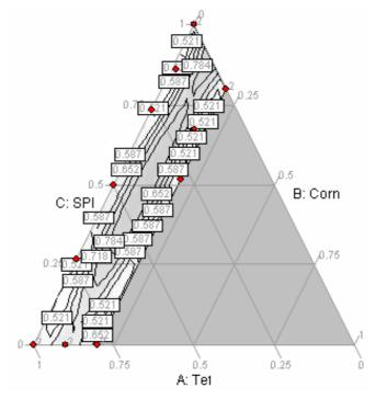
**Figure 1.** Experimental region from mixture design delimited by low and high constraints established for each component.
