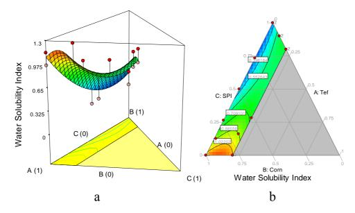
**Figure 4.** Effects of formulation on water solubility index (a) Surface response and (b) contour graph
