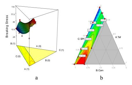
Figure 5. Effects of formulation on breaking stress (a) Surface response and (b) contour graph
